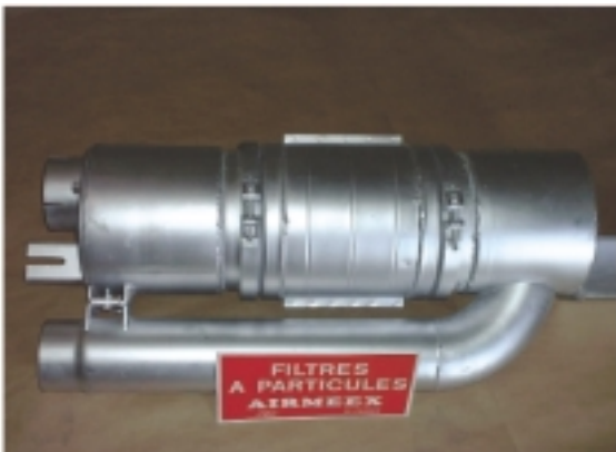
Fig. 3 View of a retrofit system for buses
