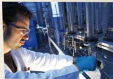
As part of the process intensification project, an experimental reactive adsorption system, aimed at combining reaction and separation operations.
