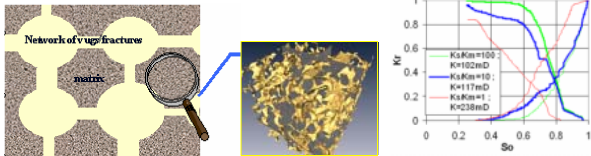
Figure 4: Schematic depiction of a dual-network and the gas/oil relative permeabilities for three different contrasts of global to matrix permeability.
