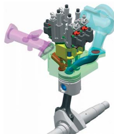
Schematic view of IFP's single-cylinder engine with Lotus VVA system
