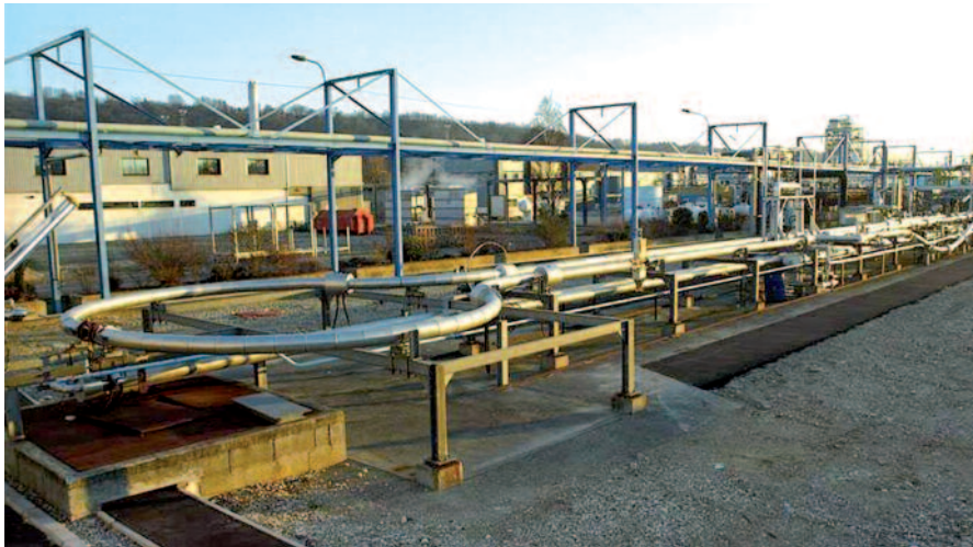
The Lyre loop high-tech tool to assess the risk of hydrate or wax formation under real conditions.
