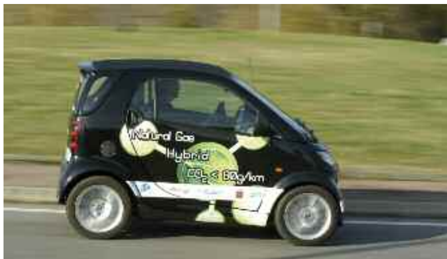
Smart Vehgan, developed by IFP in partnership with ADEME, GDF Suez, Inrets and Valeo, combining the benefits of hybridization with those associated with the use of a low-carbon fuel, natural gas.
