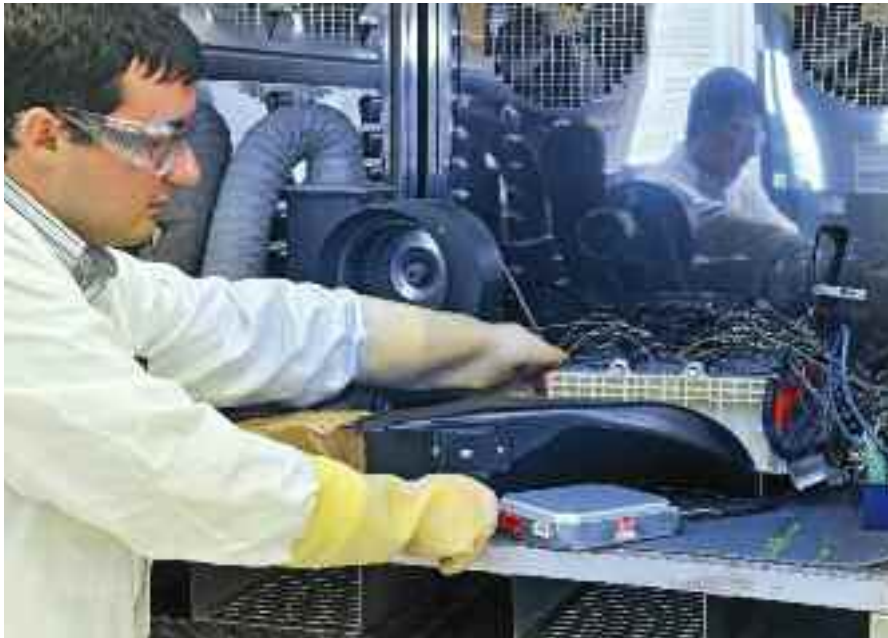
Test bench with a power of \pm 120\text{kW} to test complete battery packs in a climatic chamber ( -40^{\circ}\text{C} to +80^{\circ}\text{C} ).
