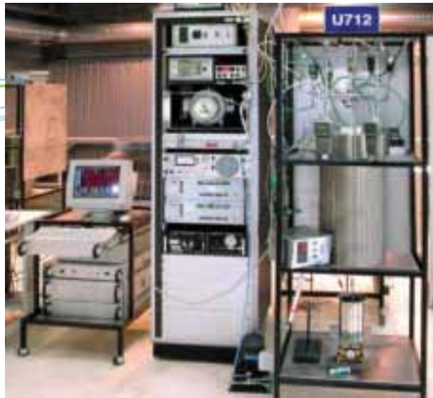
As part of the European Encap project and the ANR CLC-MAT precombustion CO 2 capture project, IFP is developing a Chemical Looping Combustion reactor and suitable metal oxides.
