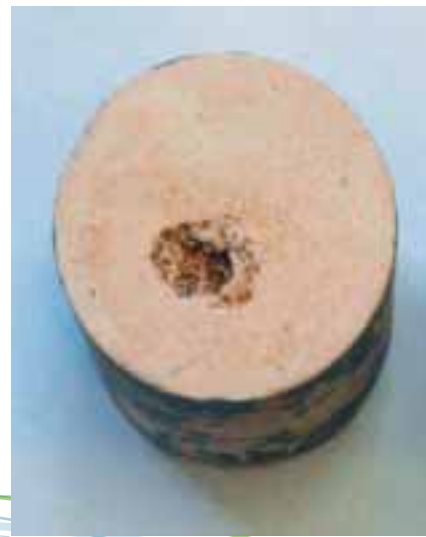
Result of an injection of CO 2 into a carbonate-containing rock.
