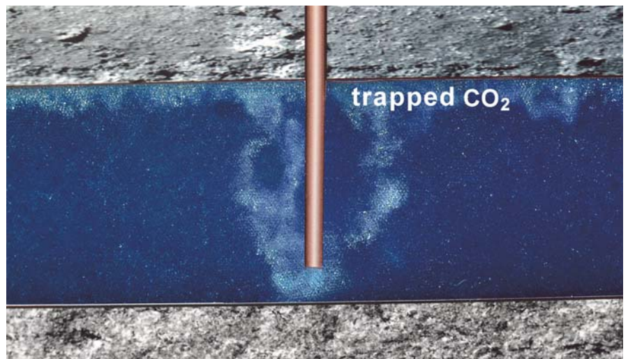
The CO 2 injected into a saline aquifer migrates in a plume through the reservoir to the cap-rock, where it is trapped.
