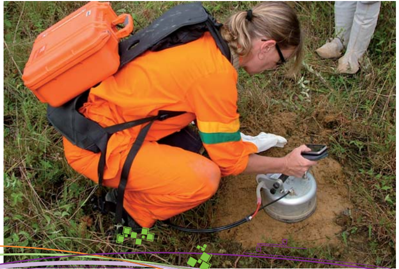
Flux chamber used to establish a geochemical baseline in the pre-injection phase.
