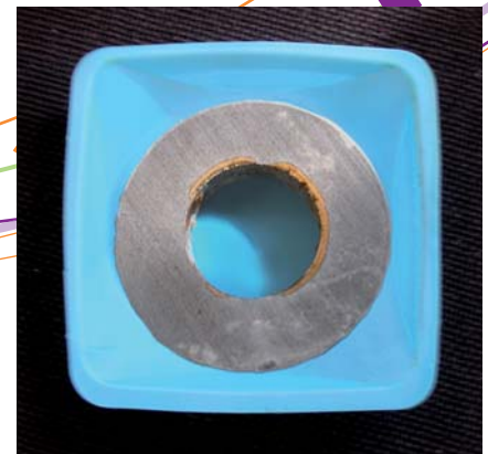
Dissolution and carbonation in the presence of CO 2 , measured in the laboratory on a cement sample.
