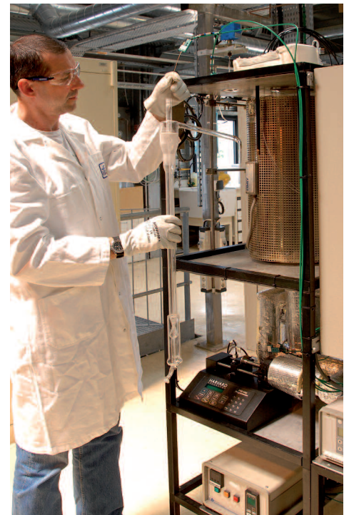
CLC batch fluidized bed reactor developed by IFP for batch studies.
