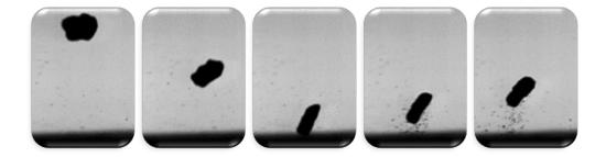
In order to describe attrition in the region of gas jets and in cyclones, these results were correlated with those measured using laboratory and pilot-scale tools, for different particle properties (diameter, density, hardness, breaking strength) and operating conditions. These correlations were then used **to estimate attrition in different regions of a CFB.**
