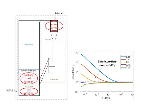
**PBM** is then used to predict, for a complete process, the evolution of particle size distribution and solid loss through attrition. This is shown in the figure below (right), illustrating the prediction of solid loss through attrition for the entire system as a function of time, for various degrees of particle breakability.
