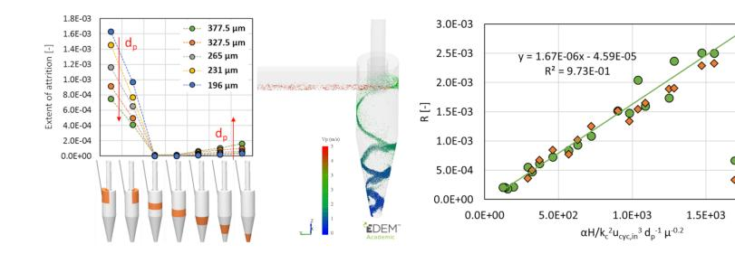
The correlations established in the different attrition regions (on the left of the figure below) were then employed in a population balance model (PBM<sup>5</sup>) in order to simulate the dynamic behavior of a circulating fluidized bed, with solid make-up.
