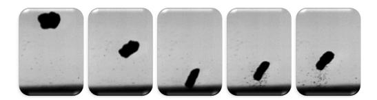
In order to describe attrition in the region of gas jets and in cyclones, these results were correlated with those measured using laboratory and pilot-scale tools, for different particle properties (diameter, density, hardness, breaking strength) and operating conditions. These correlations were then used **to estimate attrition in different regions of a CFB.**
