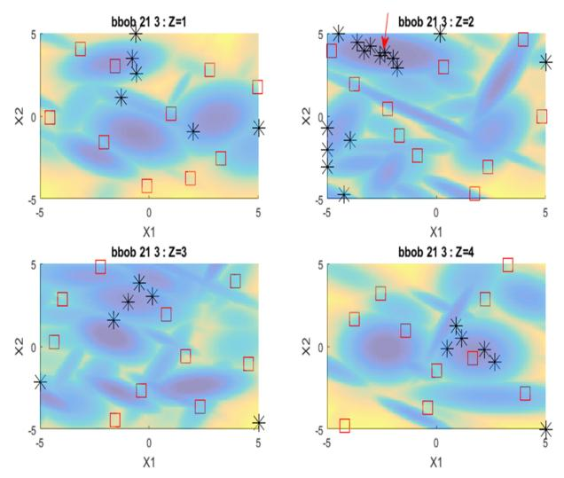
Illustration of the efficient exploration using the Cat-EGO optimization algorithm of the 4 levels of the categorical variable Z of bbob test function 21.3 from the public collection of optimization problems COCO.
