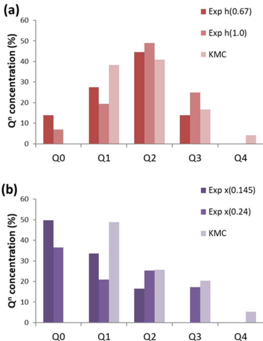
Figure 1. Comparison between kMC results using the extended set of reactions illustrated in Scheme 1 and <sup>29</sup>Si NMR experimental data with templates TMA<sup>+</sup> (a) or TPA<sup>+</sup> (b) for the different silica oligomers in terms of their Si-O-Si connectivity expressed as Q<sub>n</sub>.
