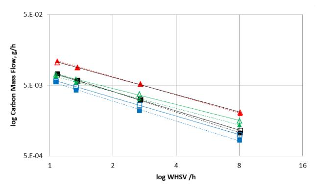
Figure 2: Carbon flows at 340°C: Ethylene (square), Diethyl Ether (triangle). Ethanol/acetaldehyde ratio: 3.6 (black and red); 2.5 (blue and green). The lines are trend curves (experimental values: dotted lines, filled symbols - simulated values: solid lines, unfilled symbols) [1]
