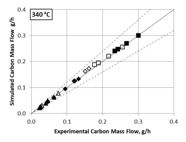
Figure 3: Parity graphs at different WHSV at 340°C: ethanol (square), acetaldehyde (triangle), butadiene (diamond shape). Ethanol/acetaldehyde ratio = 3.6 (filled symbol); 2.5 (unfilled symbol). Dotted curves,  $\pm 20\%$  error. [1]
