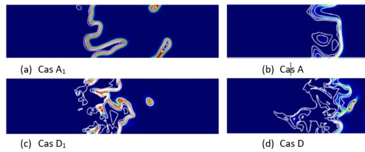
2D sections extracted from 3D simulations representing heat release rate and temperature isosurfaces
