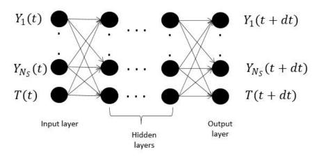
Illustration of the neural network resolution approach for the combustion of H2
