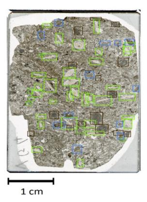
Figure 2: Automated microfossil detection on a thin rock section. Each rectangle generated by the algorithm defines a zone containing a microfossil. Its color corresponds to the most likely species according to the model (e.g., green for nummulites, brown for alveolinids)
