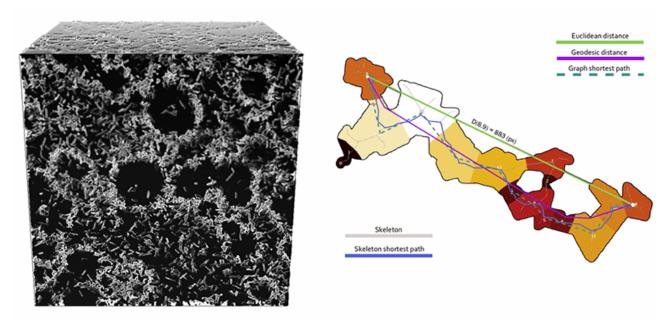
On the left, numerical simulation of the microstructure of a porous material. On the right, illustration of a tortuosity operator, ratio of the lengths of paths between two points "as the crow flies" (Euclidean distance) and constrained by the porous network (geodesic distance).
