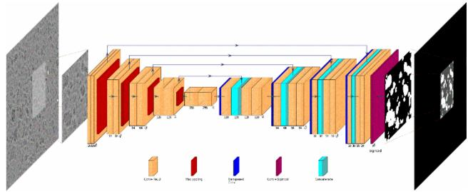
Illustration describing the semantic segmentation of a microscopic image into different zones of porosity heterogeneity with a convolutional neural network. The output image is reconstituted from random patches extracted from the input image.
