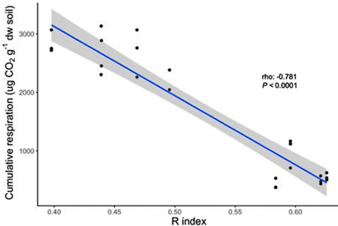
Figure 1: Determination of the CO<sub>2</sub> generated by SOM mineralization (R-Index: descriptor of SOC stability obtained from the Rock-Eval® analysis) [4]
