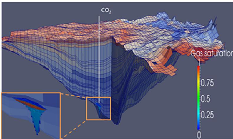
Figure 1: CO<sub>2</sub> injection modeling in a potential basin – combination of basin and reservoir modeling tools
