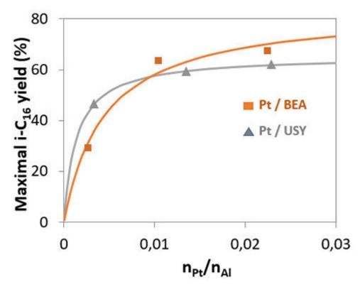
Figure 1: Change in the maximum isomerisation yield (a descriptor of the selectivity in isomerisation, during the hydroconversion of n-hexadecane, according to the ratio between metallic sites (Pt) and Brønsted sites (Al) for two zeolites (HBEA and HUSY) [1].
