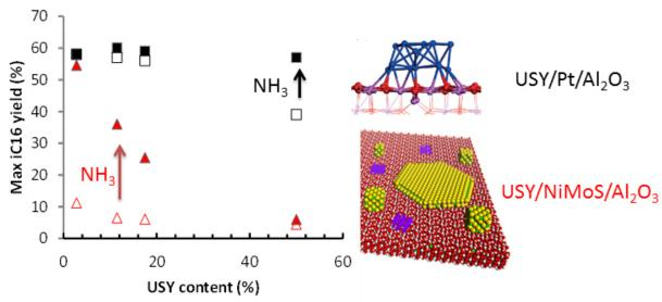
Figure 2: Comparison of Pt-based (black) with Ni/MoS2 catalysts (red). The concentration of acid sites has been modified by varying the USY zeolite content in the extruded product. The figure shows the maximum yield in iC16, in the presence (filled symbols) or absence (empty symbols) of an ammonia inhibitor.
