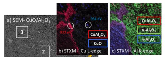
Figure: a) SEM image of a CuO/Al2O3 oxygen carrier material after 50 cycles, and STXM 10x10 ?m mapping of the area indicated by the yellow square; b) at the copper L-edge; c) at the aluminium K-edge.
