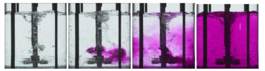
Figure 1: Illustration of the mixing in water mechanism, at several points in time (photographs), from injection (a) through to complete mixing (d)
