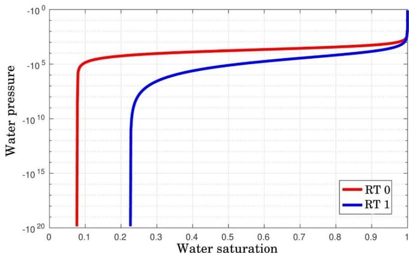
Figure 1 : An example of pressure as a function of water saturation obtained with a Van Genuchten-Mualem-type model for two types of rock Position: RT0 and RT1.
