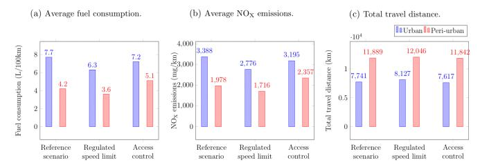
Figure 4: Fuel consumption, NOx emissions and traffic flow for each of the three control strategies.
