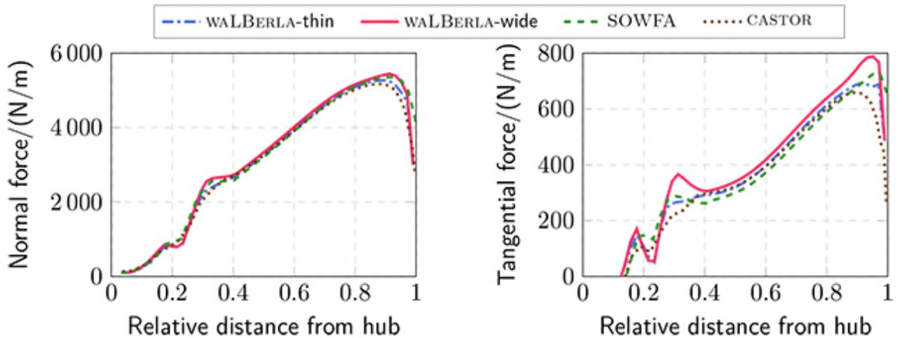
Figure 2: Distribution of normal (left) and tangential (right) forces along the blade.
