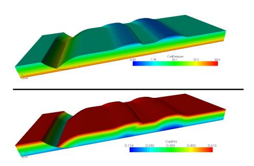
Flow calculation in basin simulation (TemisFlow ArcTem simulator). The mesh includes faults and evolves during simulation
