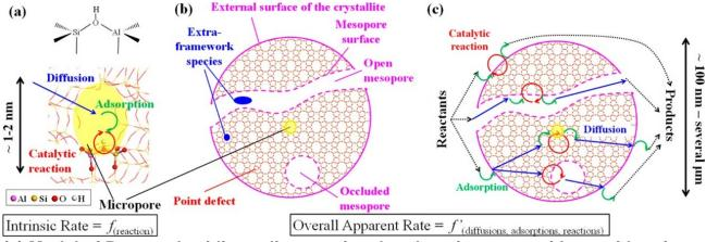
(a) Model of Brønsted acidic zeolite, restricted to the micropore, with consideration of diffusion, adsorption, and reactions steps. (b) Scheme of defect and finite size nature of an intricate zeolite crystallite. A spherical crystallite model is arbitrarily chosen. (c) Integration of the variety of sites and of steps for the definition of the overall apparent reaction rate. Copyright 2023 American Chemical Society
