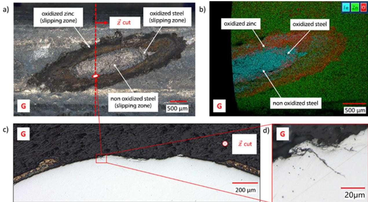
Figure 2: single interrupted fretting test on galvanized wires
