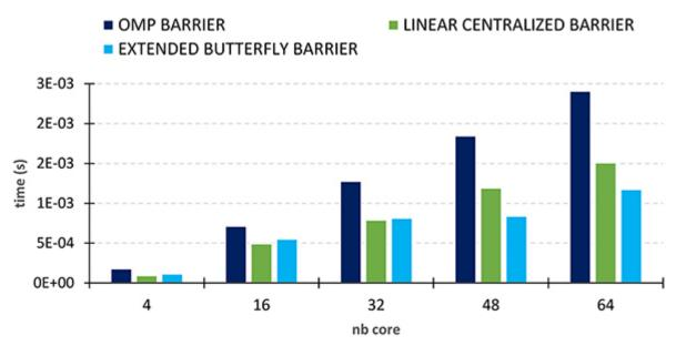
Figure 2: Result of barrier synchronization times on the AMD Milan processor.
