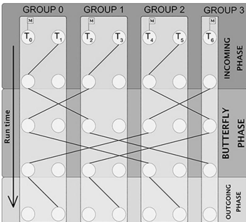
Figure 1: Illustration of notification exchanges between cores in the Extended Butterfly barrier with 7 cores or threads. The dark lines symbolize the sending of notifications from one core to another. The barrier consists of 3 steps: an input step, a step in Butterfly and an output step. Only the cores represented with a flag are authorized to enter in the Butterfly phase while their partner waits for their output phase notification.
