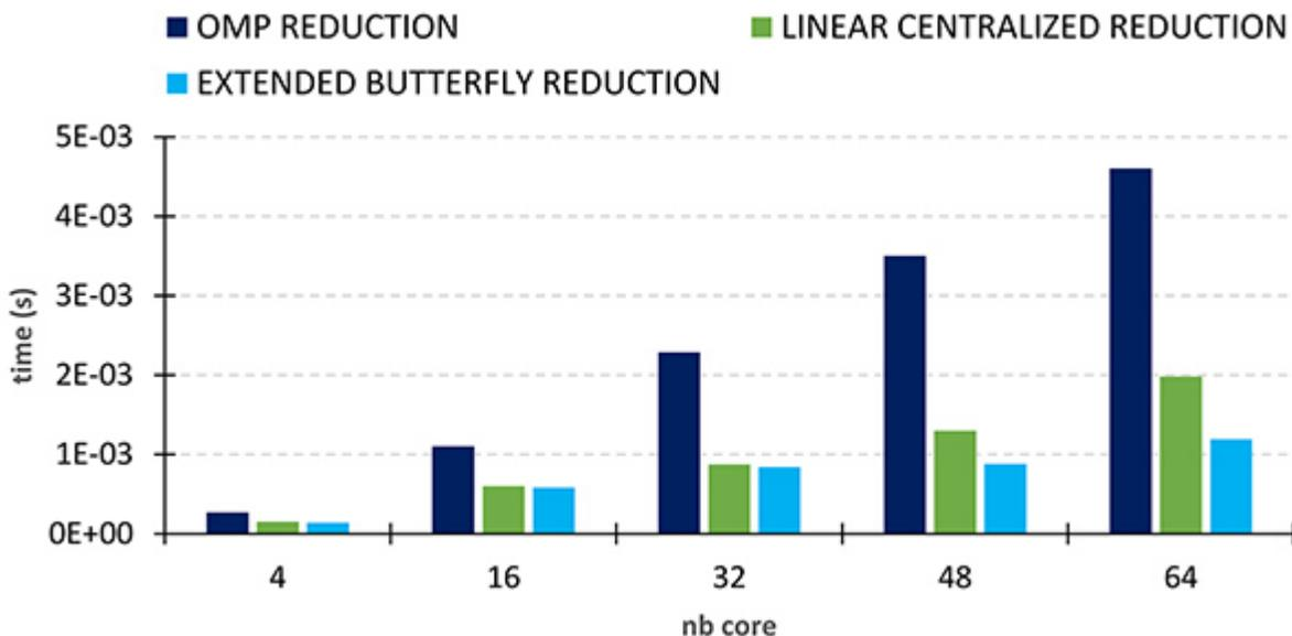
Figure 3: Result of reduction times on the AMD Milan processor.
