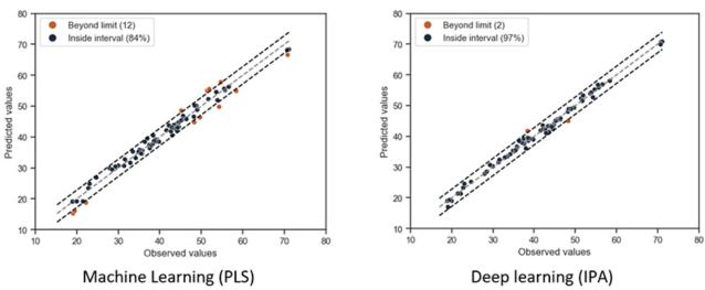
Figure 2: Parity plot – Middle distillates (reduced spectral range of 4,500-1,200 cm-1)
