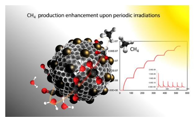
Figure 3: Representation of the platinum-on-TiO2 catalyst, reagents and products of the photoreduction of CO2. The graph illustrates the evolution of the cumulative quantity of CH4 produced and its derivative as function of time.
