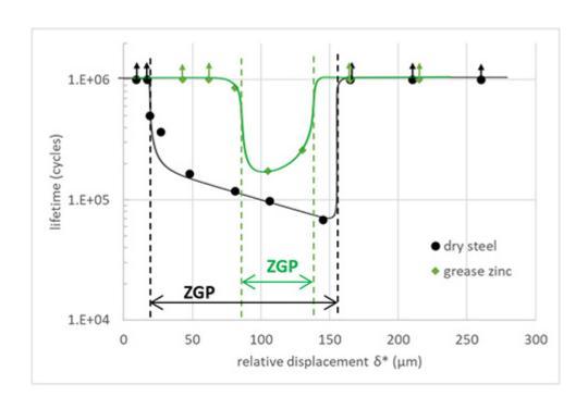
Figure 3: Fretting fatigue curves for dry contact between steel wires (black) and greased contact between galvanized wires (green). Load under constant fatigue and force conditions Relative slip between wires on the x-axis and lifespan on the y-axis. The combination of zinc and grease significantly increases lifespan. ZGP: critical damage zone in partial slip conditions
