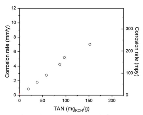
Figure 2: Influence of TAN on the corrosion rate of AISI 1018 carbon steel during immersion tests at 220°C (mixture of rapeseed oil and oleic acid)
