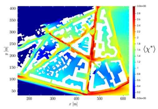
Figure 1: Example of pollutant concentration map simulated by the calculation chain described in [1] for a neighborhood in Issy-les-Moulineaux, near Paris.
