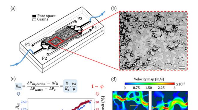
Figure 1 - (a) Illustration of the micromodel used. P1/P2/P3 and P4 correspond to pressure measurements.
