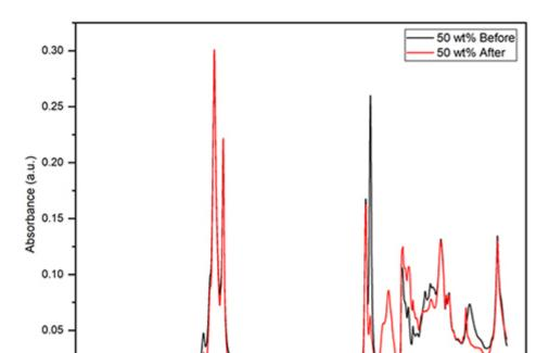
Figure 3: Infrared spectrum of an acidic vegetable oil before and after corrosion test
