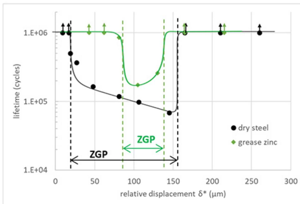
Figure 3: Fretting fatigue curves for dry contact between steel wires (black) and greased contact between galvanized wires (green). Load under constant fatigue and force conditions Relative slip between wires on the x-axis and lifespan on the y-axis. The combination of zinc and grease significantly increases lifespan. ZGP: critical damage zone in partial slip conditions
