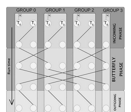
Figure 1: Illustration of notification exchanges between cores in the Extended Butterfly barrier with 7 cores or threads. The dark lines symbolize the sending of notifications from one core to another. The barrier consists of 3 steps: an input step, a step in Butterfly and an output step. Only the cores represented with a flag are authorized to enter in the Butterfly phase while their partner waits for their output phase notification.
