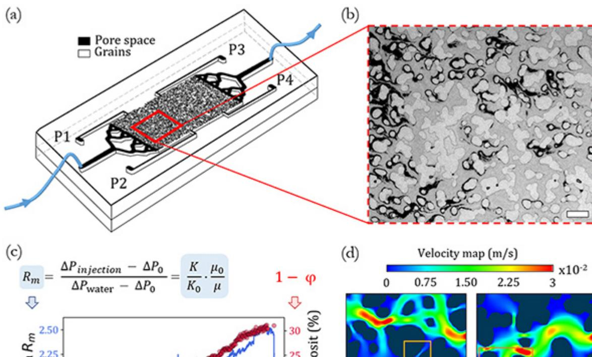
Figure 1 - (a) Illustration of the micromodel used. P1/P2/P3 and P4 correspond to pressure measurements.
