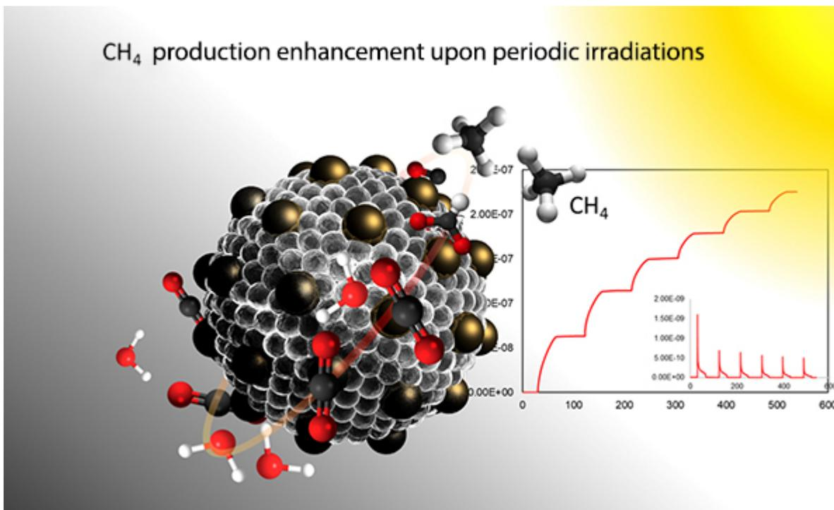
Figure 3: Representation of the platinum-on-TiO<sub>2</sub> catalyst, reagents and products of the photoreduction of CO<sub>2</sub>. The graph illustrates the evolution of the cumulative quantity of CH<sub>4</sub> produced and its derivative as function of time.
