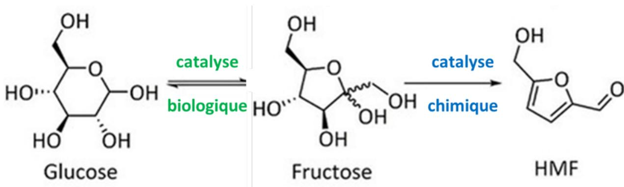
Figure 1. The conversion of glucose into HMF
