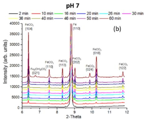
Figure 6: In situ XRD analysis of an X65 carbon steel coupon at 80°C at 0.54 bar of CO<sub>2</sub>, flowing at a velocity of 0.1 m/s through a flow cell at pH 7. Individual diffraction peaks evolving with time over the course of a test duration of around 1 hour [3].
