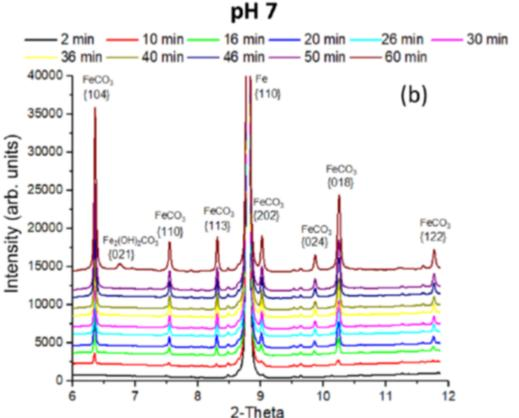
Figure 6: In situ XRD analysis of an X65 carbon steel coupon at 80°C at 0.54 bar of CO2, flowing at a velocity of 0.1 m/s through a flow cell at pH 7. Individual diffraction peaks evolving with time over the course of a test duration of around 1 hour [3].
