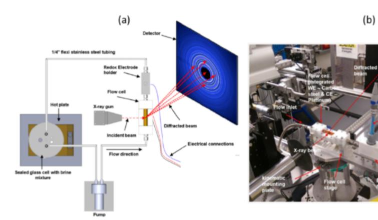
Figure 5:(a) Illustration and(b) configuration of the flow cell used on the Diamond Light Source beamline (Oxford) [3]
