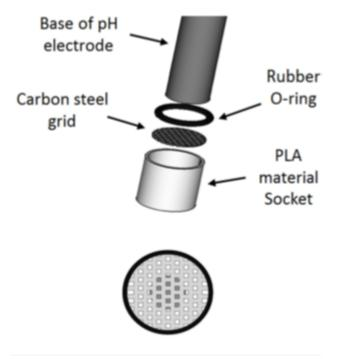
Figure 1: pH electrode diagram [1]
