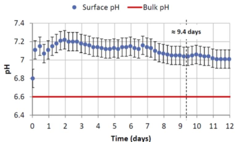
Figure 2: Surface pH measurement conducted for a pH of 6.6 measured in a full bath (a long way from the sample surface) over a test period of 12 days at 80°C at 0.54 bar of CO<sub>2</sub> [1]
