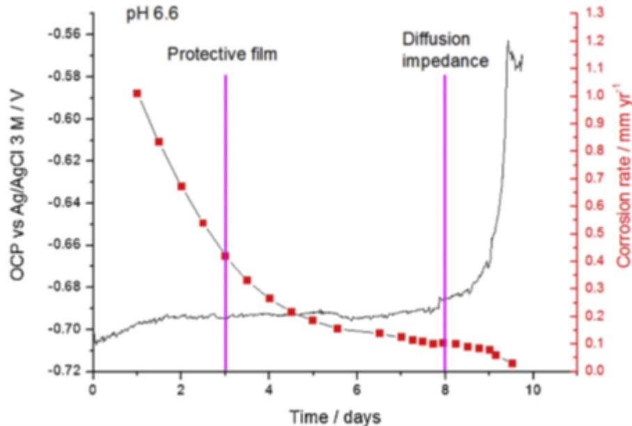
Figure 3: evolution of Open Circuit Potential and corrosion rate as a function of immersion time for a bulk bath pH of 6.6 (interfacial pH of 7) at 80°C and 0.54 bar of CO<sub>2</sub> [2]
