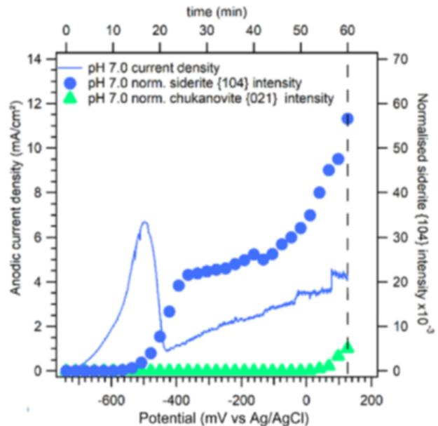
Figure 7: Normalized FeCO<sub>3</sub> (104) and Fe<sub>2</sub>(OH)<sub>2</sub>CO<sub>3</sub> (021) lattice plane intensity during potentiodynamic polarization in the anodic domain of the X65 carbon steel coupon in an 80 °C and 3.5 wt% NaCl solution saturated with CO<sub>2</sub> at 0.54 bar pCO<sub>2</sub>, flowing at a velocity of 0.1 m/s through the flow cell at pH 7 [3].
