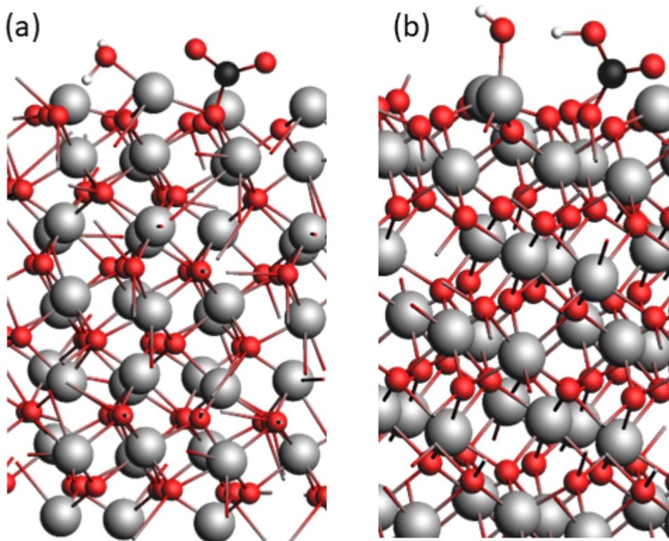
Figure 1:(a) CO<sub>2</sub> adsorption on the Cr<sub>2</sub>O<sub>3</sub> surface, with crystallographic orientation (0001), where a water molecule is pre-adsorbed. (b) formation of a bicarbonate anion. Color code: oxygen (red), chromium (gray), carbon (black), hydrogen (white).
