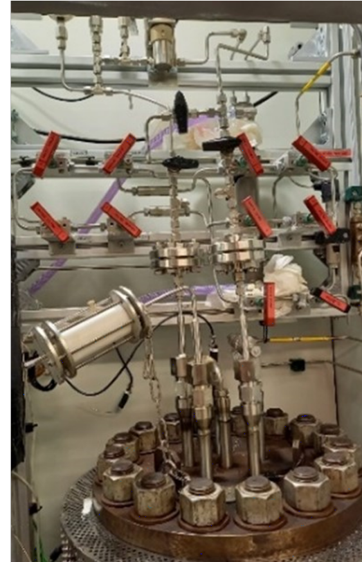
Figure 5: Illustration of the set-up for electrochemical monitoring with deposit formation via heat exchange on the corrosion test loop.
