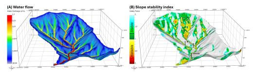
Fig. 2: (A) Numerical hydro-sedimentary modeling using the ArcaDES code, with calculation of the torrential water flow (flow rate, height and speed) at the peak of the storm, (B) Calculation of the stability factor of the slopes of the Viévola valley as a function of the stresses induced by the torrential flow.
