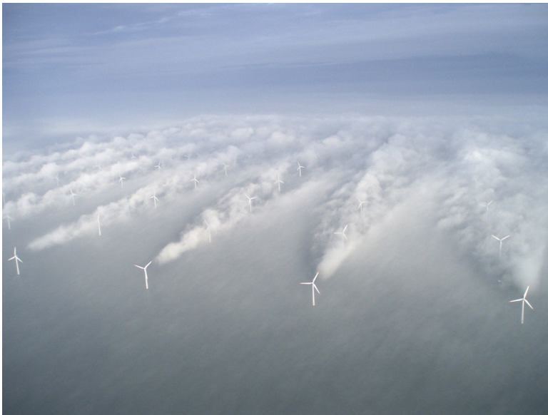
Figure 1: Visible wake effects on the Horns Rev 1 offshore wind farm - copyright Vattenfall.
