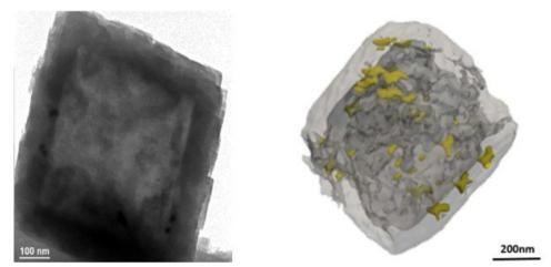
Figure 5: TEM image of a hollow Beta zeolite crystal containing encapsulated platinum nanoparticles (left); reconstitution of a crystal using 3D tomography (right).
