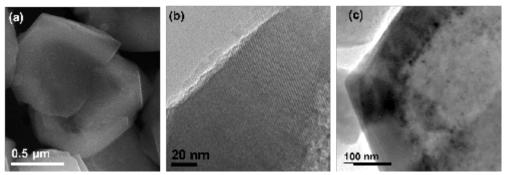
Figure 3: Microscopic observation of a hollow Y zeolite crystal: MEB visualization of a more marked contrast at the wall (a); TEM images showing the zeolite network visible in the wall (b) and on metal particles inserted within the walls (c).
