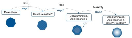
Figure 2: Illustration of hollow Y zeolite preparation based on a 3-step process.
