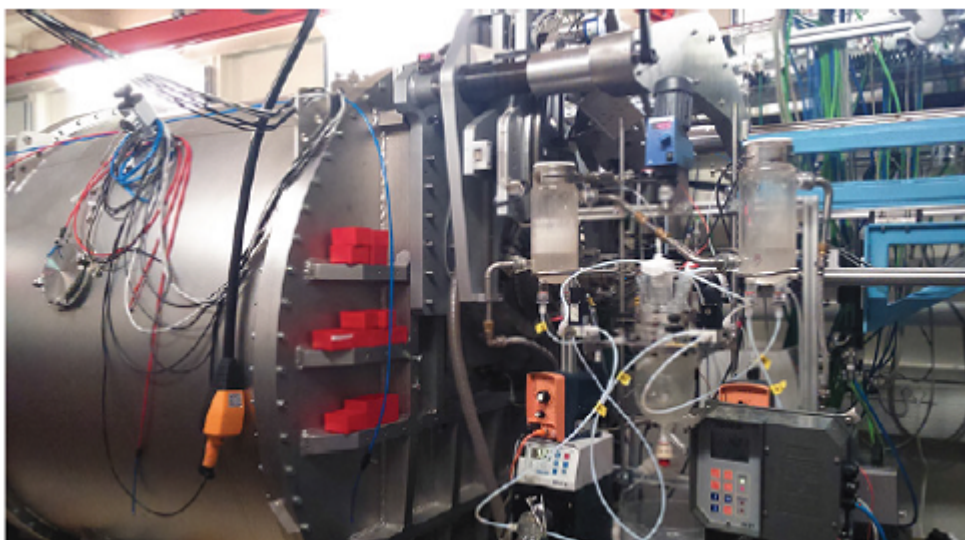
Installation of the synthesis system on the SWING beamline of the synchrotron SOLEIL.
