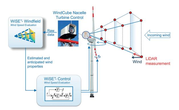
Real-time knowledge of incoming wind provided by lidar enables wind turbine and farm control and production optimization. IFPEN develops various control solutions in this field:
