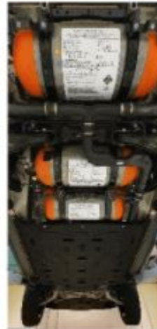
FC vehicle on the chassis dynamometer / FC vehicle tanks
