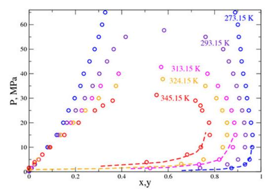
Example of pressure-composition diagrams generated using molecular simulation, for a binary sulfur dioxide / nitric oxide system.
