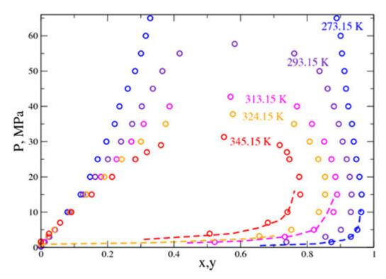
Example of pressure-composition diagrams generated using molecular simulation, for a binary sulfur dioxide / nitric oxide system.
