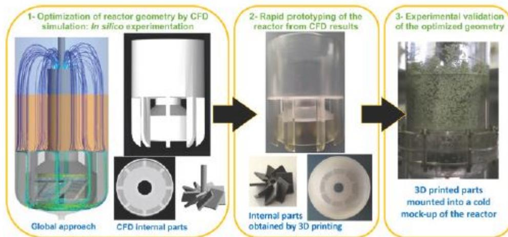
Three-phase stirred tank reactor: from CFD (left\*) to technological reality (right).
