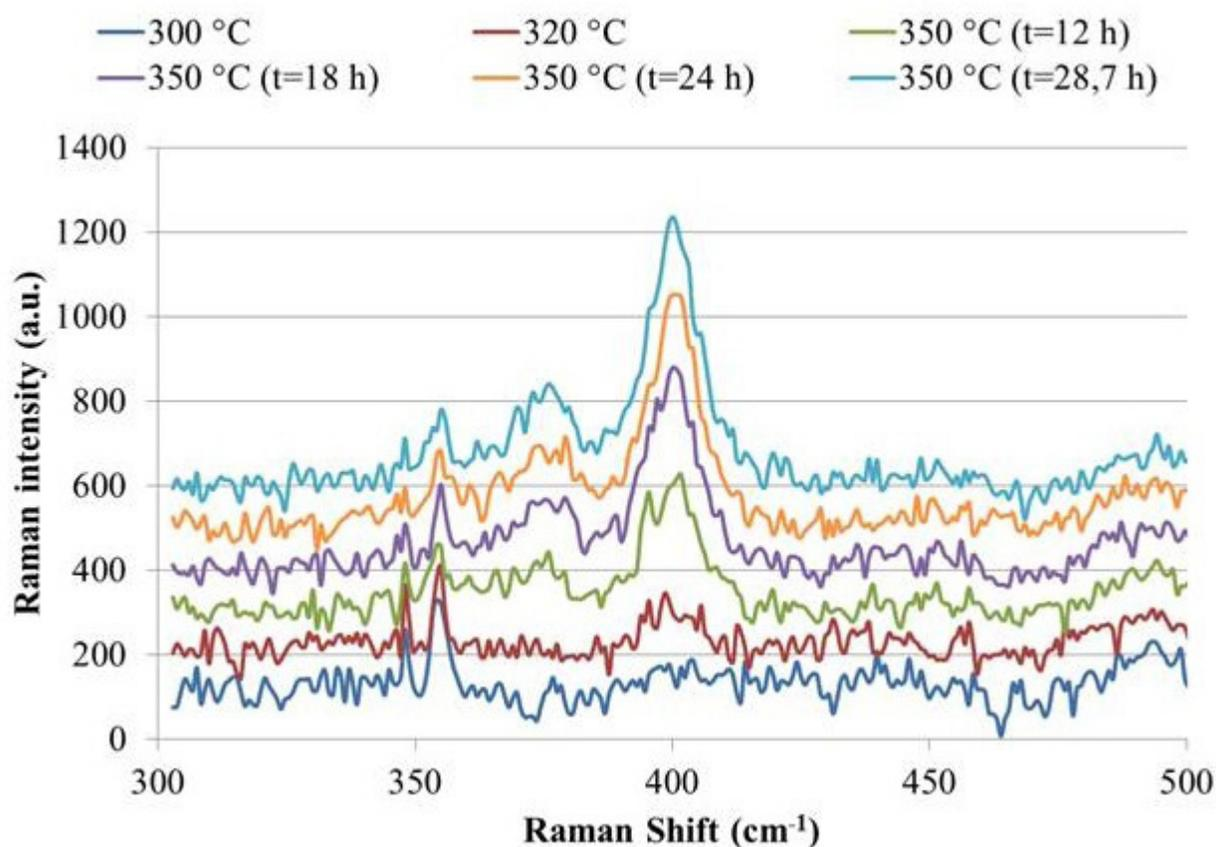
Temporal follow-up of the active phase (MoS<sub>2</sub> at 375 and 400 cm<sup>-1</sup>) during the activation of a calcined CoMoP catalyst under a (diesel + DMDS) mixture
