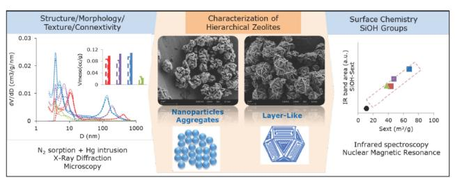
Morphological, textural and surface characterization of different zeolites with hierarchized porosity used for xylene separation.
