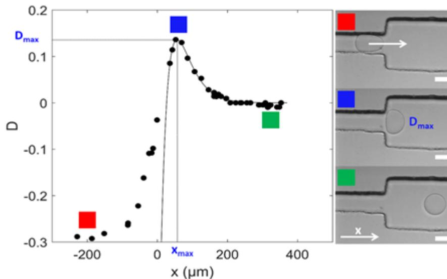
Deformation of a droplet passing through a microfluidic restriction (at  $x = 0$ ).
