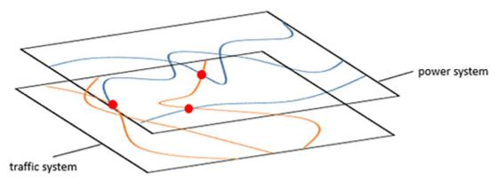
Principle of overlaying the traffic system diagram and the electrical network diagram used in the optimization model
