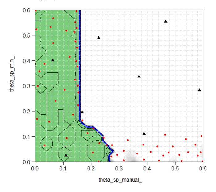
For two control parameters, estimation (in green) of the NH3 emission standard compliance set (initial simulated points in black, points added via the iterative method in red).
