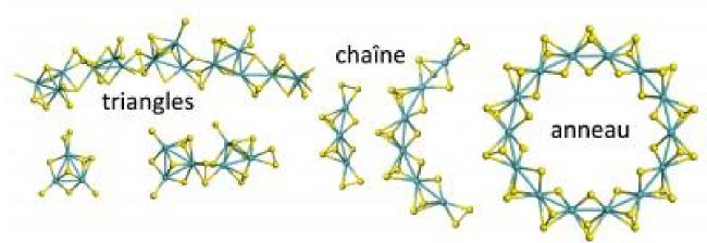
Various amorphous MoS3 phase nanoclusters identified by quantum simulations.
