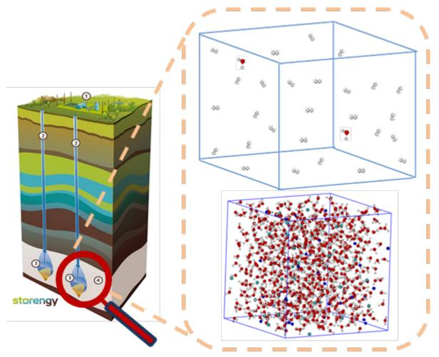
**Principle of the methodology:** the phase equilibrium occurring within a geological storage site is determined via Monte Carlo-type molecular simulations. The equilibrium data generated can then be used to calibrate the empirical laws used by operators.
