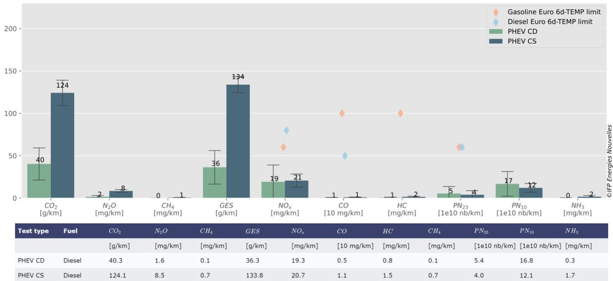
Figure 22 : Comparison of the mean emissions in CS and CD mode of the diesel plug-in hybrid vehicle selected on the experimental protocol.
