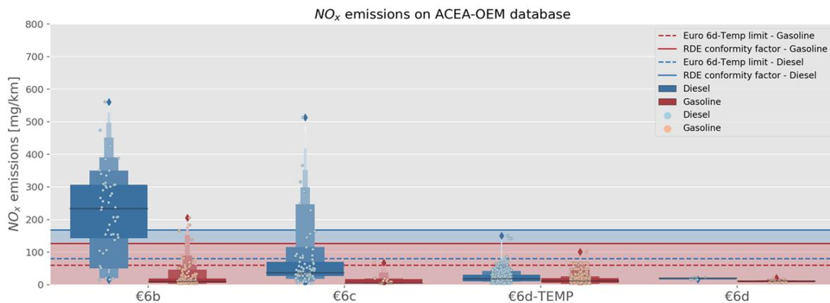
Figure 4 - Manufacturer's NO<sub>x</sub> emissions data on RDE. Sources: ACEA and JAMA
