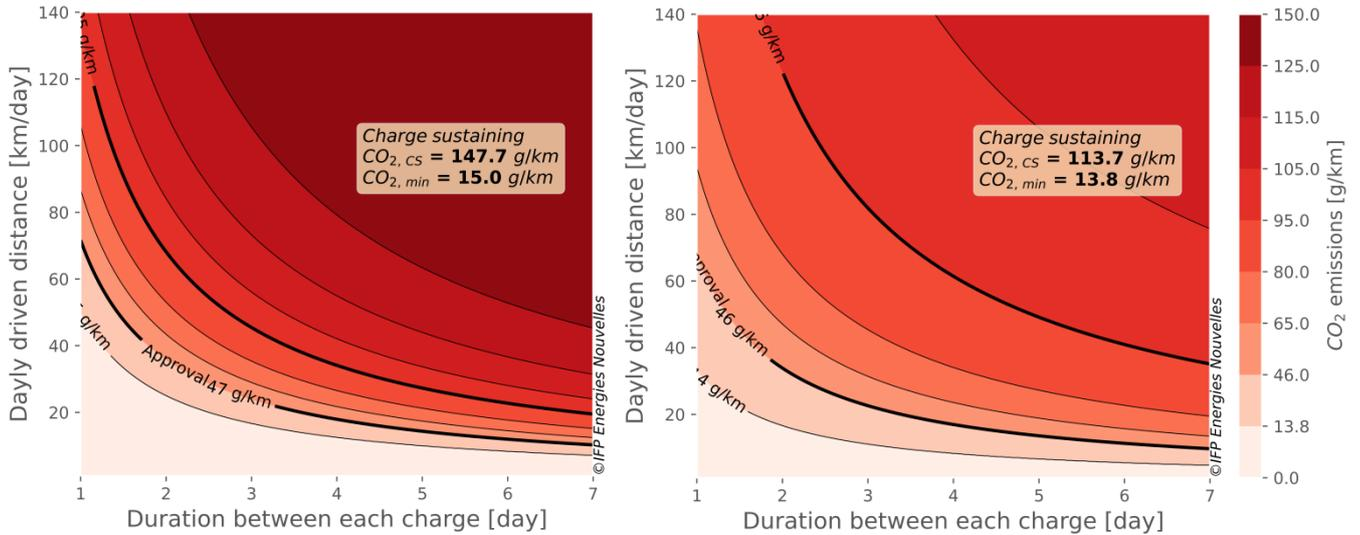
Figure 23 - CO<sub>2</sub> emissions from PHEV gasoline (left) and diesel (right) vehicles, depending on the frequency of recharging and the length of daily trips. The approved CO<sub>2</sub> score is also shown (Approval). Tests on a climatic chassis dynamometer are excluded from the considered scope.
