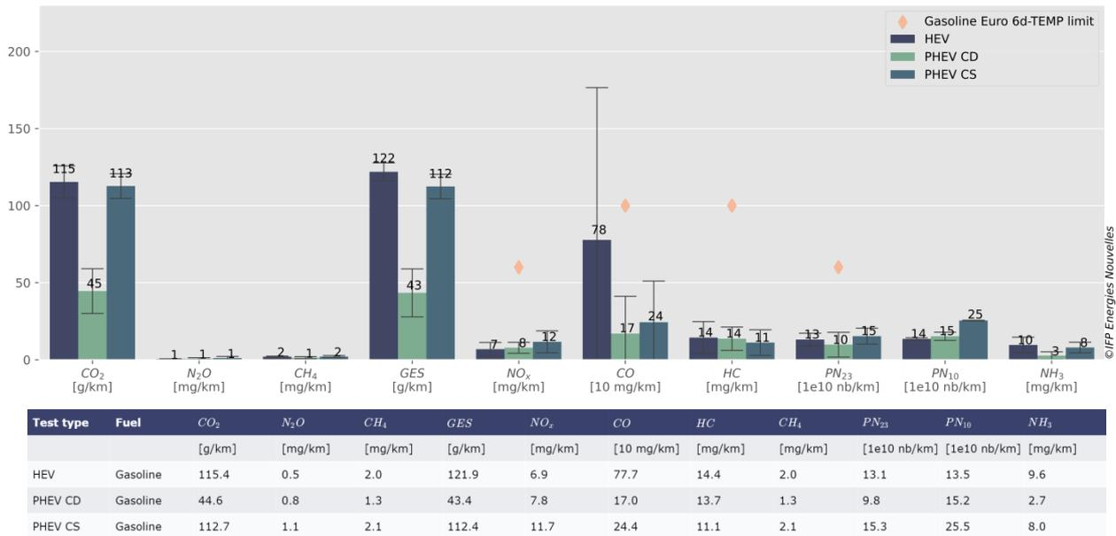
Figure 19 : Comparison of the average emissions of the non-rechargeable hybrid (HEV) and plug-in hybrid vehicle selected on the experimental protocol.
