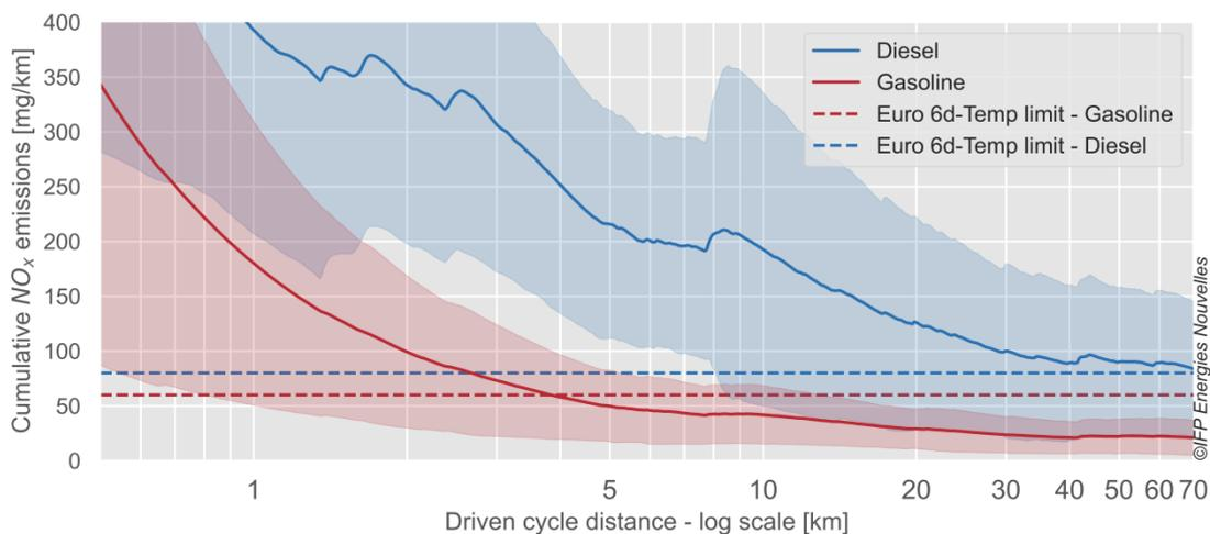
Figure 27 : Evolution of cumulative NO<sub>x</sub> emissions as a function of the distance on the RDE test
