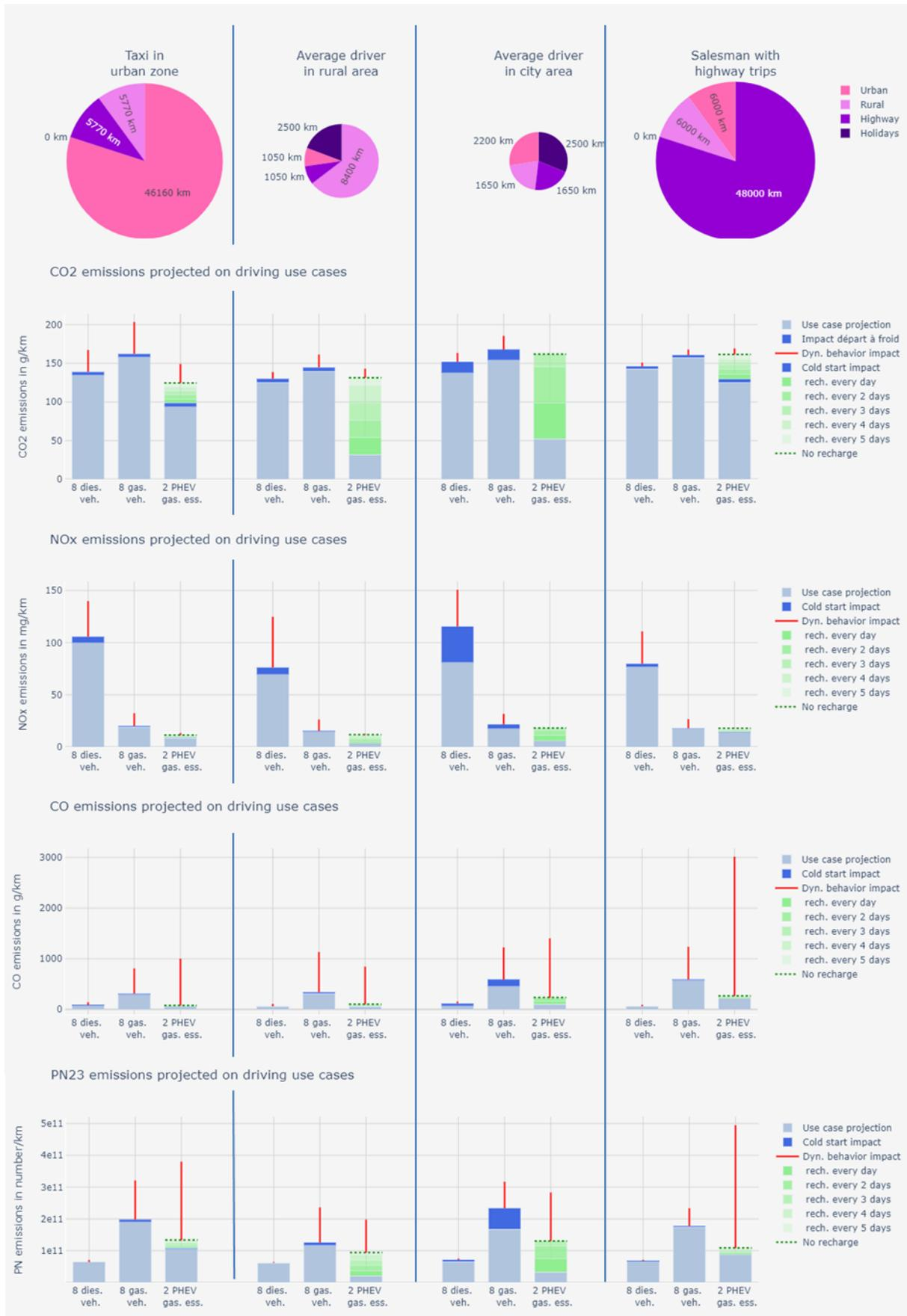
Figure 29 : Comparison of average emissions of CO<sub>2</sub>, NO<sub>x</sub>, CO and PN<sub>23</sub> projected on uses for diesel and gasoline combustion vehicles, and gasoline PHEV vehicles
