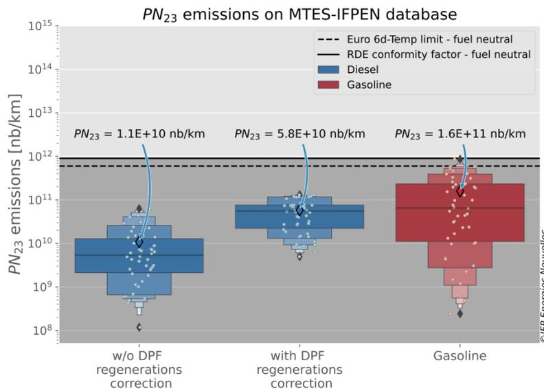
Figure 11 : Comparison of number of particulate emissions over 23 nm from gasoline and diesel vehicles over the full scope of the study
