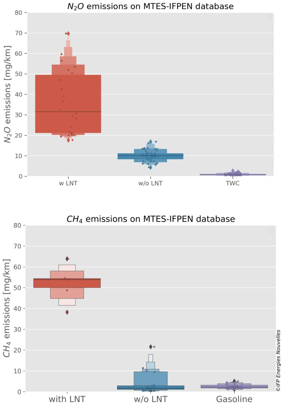
Figure 33 : Comparison of N<sub>2</sub>O and CH<sub>4</sub> emissions according to the types of pollution control of diesel and gasoline vehicles.
