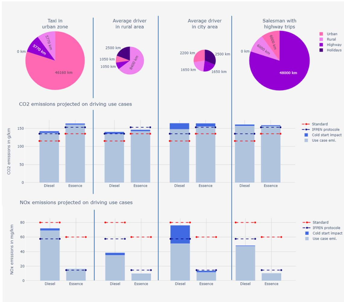
Figure 30 : Comparison of CO<sub>2</sub> and NO<sub>x</sub> emissions projected on uses for gasoline and diesel compact SUV vehicles (GV3 and DV3)
