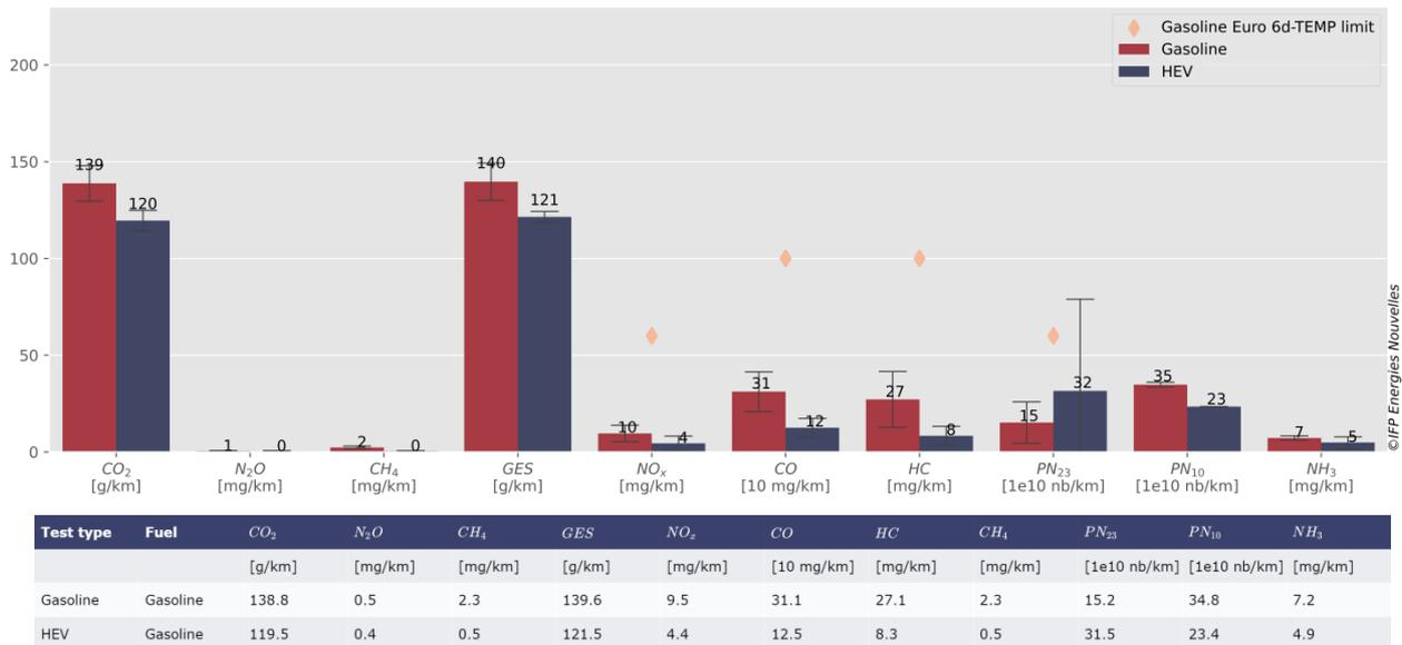
Figure 18 : Comparison of the average emissions of the gasoline and hybrid vehicle selected on the experimental protocol.
