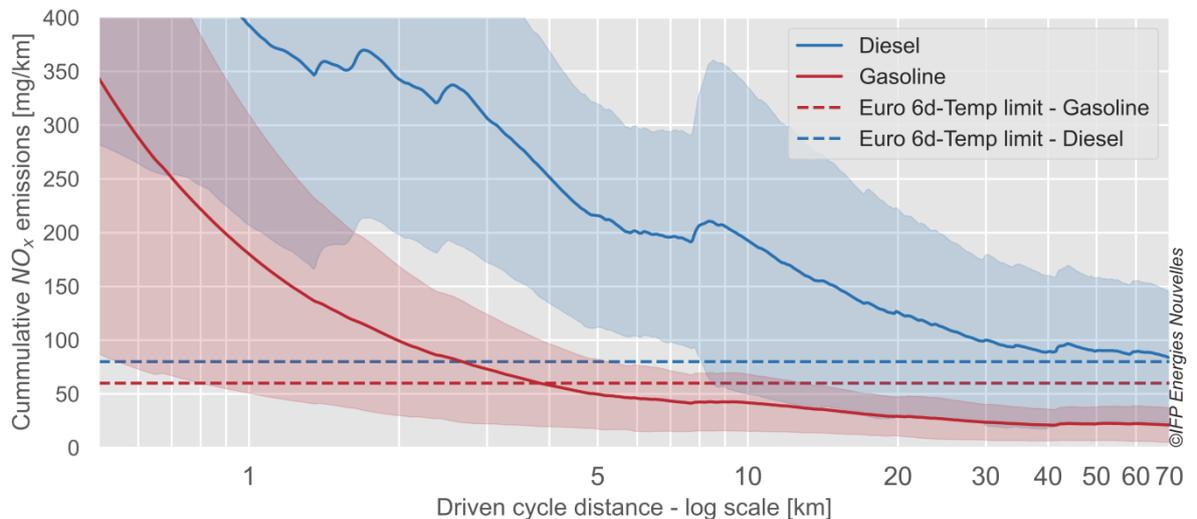
Figure 3 : Comparison of the evolution of cumulative NO<sub>x</sub> emissions as a function of the distance on the RDE test between gasoline and diesel vehicles (thick lines). The colored areas represent the standard deviation.
