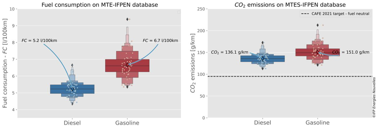
Figure 7 : Comparison of CO<sub>2</sub> emissions and fuel consumption of gasoline and diesel vehicles over the full scope of the study
