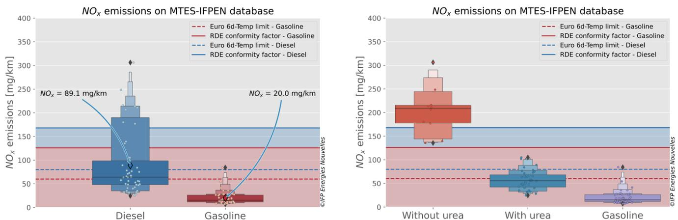
Figure 10 : Comparison of  $NO_x$  emissions from gasoline and diesel vehicles over the full scope of the study
