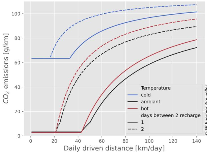
Figure 25 : Impact of the test temperature on CO<sub>2</sub> emissions according to use for PHEV gasoline SUV : comparison of RDE tests on cold (-2 °c), nominal (22 °c) and hot ( 35 °c). Road tests are excluded from the considered perimeter to isolate the temperature effect on identical routes.
