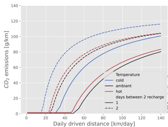
Figure 26 : Impact of test temperature on CO<sub>2</sub> emissions as a function of use. The scope considered consists of the RDE and WLTC tests on a climatic chassis dynamometer (gasoline on the left, diesel on the right).
