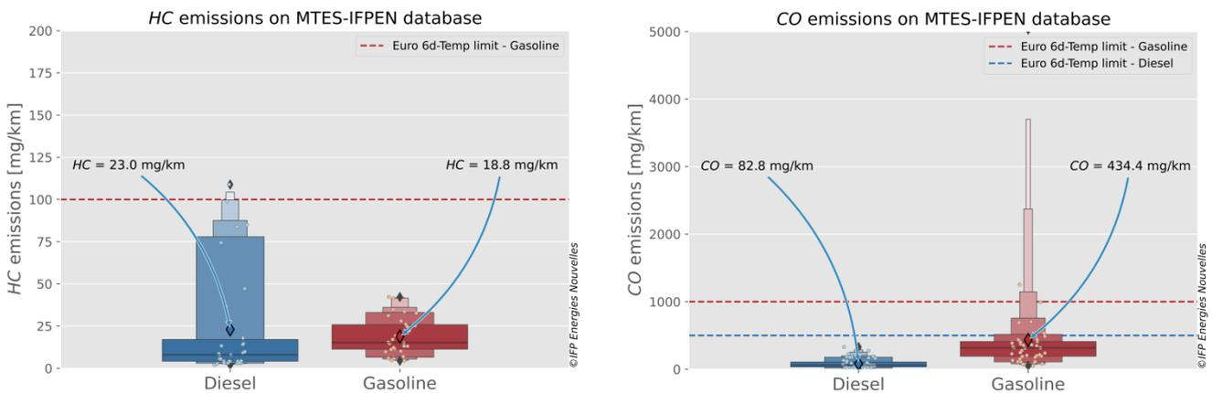
Figure 12 : Comparison of *HC* and *CO* emissions from gasoline and diesel vehicles on: laboratory tests for *HC*, the full scope of the study for *CO*
