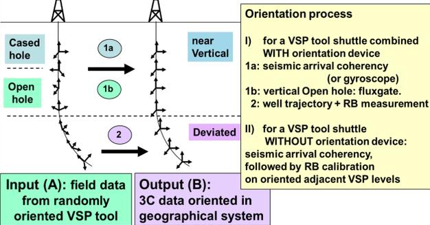
The orientation process from VSP field measurements consists in three successive rotations, sketched below, starting with the RB angle from the inclinometers:
