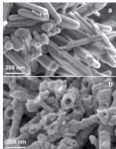
Scanning Electron Microscope images of ZnO particles before (a) and after sulfidation (b).
