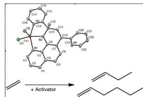
N,N,N ligands and corresponding iron(III) complexes. Application to ethylene oligomerization.
