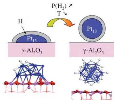
Model of the reconstruction of a Pt<sub>13</sub> aggregate on a  $\gamma$ -alumina substrate in H<sub>2</sub> atmosphere.
