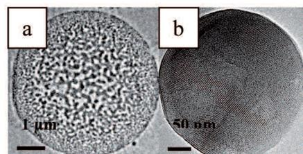
a) Particle with a hierarchized porosity, mesoporous at the edges, macroporous in the center.
