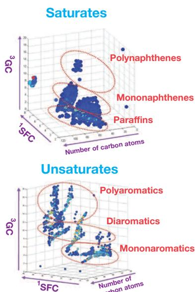
3D chromatograms produced by analysis of a vacuum distillate by SFC/GC2D-HT coupling.
