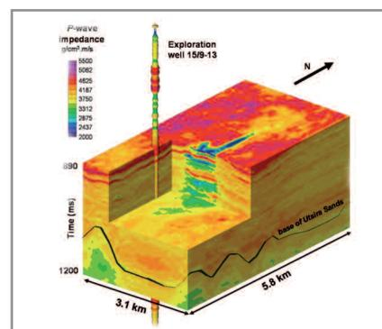
3D view of the distribution of P wave impedance obtained following seismic inversion of data acquired in 2006. CO<sub>2</sub> is identified by lower impedance values (blue and green colors) inside the reservoir (as per Clochard et al. *First Break* 2010).
