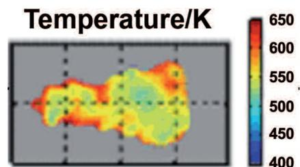
Image of the temperature in a non-reactive diesel jet obtained by laser induced fluorescence.
