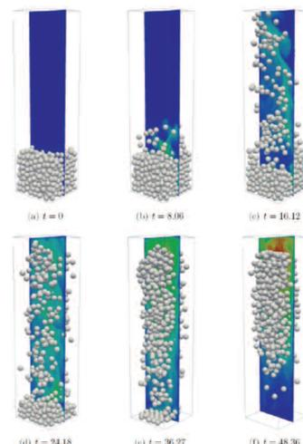
Re-suspension of 500 spherical catalysts by natural convection: temperature evolution over time.
