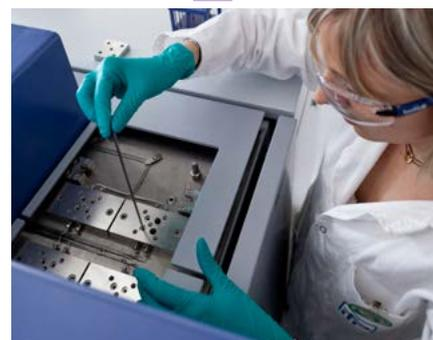
Loading of reactors on HTE equipment.
